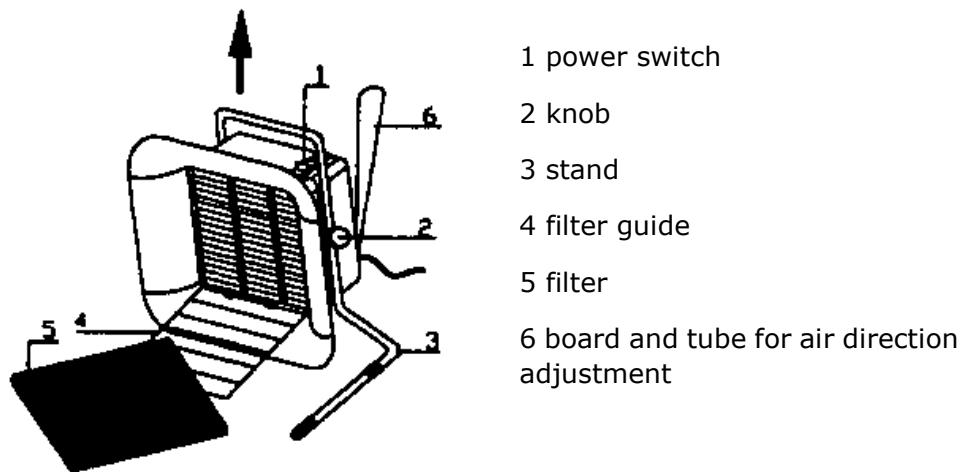
As for the desktop smoke absorber, be sure to make it stable on the desk. The angle can be adjusted to achieve the optimum smoking effect.
