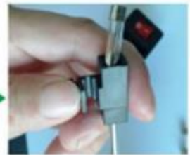
3. Remove the damaged fuse with a screwdriver
